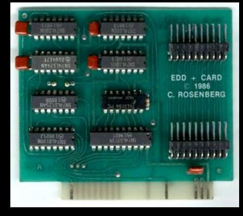
Duplicator (EDD) software. This card is a little bit like a mid-1980s Kryoflux. Nowhere near the resolution, and it runs in a 1MHz machine, but it read bits faster and in more "raw" format than the Disk II card.
